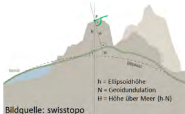
Figure 4. Influence of the geoid on the horizon of the instruments and on the effective altitude above sea level; not shown to scale.
